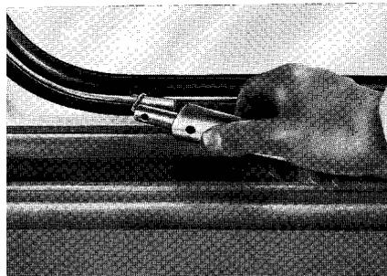
It is easier to insert the filler section, especially around the corners, by applying light alternating pressure on the tool and angling it slightly. After the eyelet in the tool has been slipped along the entire length of the channel, it is then lifted out of its groove.
